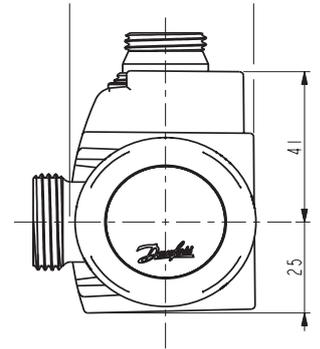
VHS-DV Eckventil (RAX-Fühler, an Position 3)
