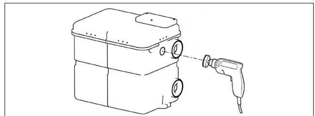
**CAUTION!** Do not damage the raised and flat face ! and push the enclosed plug-in seals into the opened connection branches.
