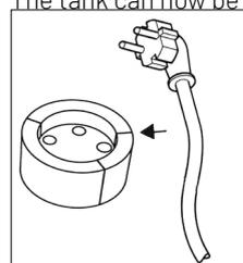
4. Pull the pump cable with the plug through the Ø 70 mm hole in the cover. Swing open the seal plug, insert the pump cable and push the plug into the provided hole in the cover. The cable in the tank must be so short that the float moves free. For the outer cable length think about the installation of the cover and necessary maintenance.
